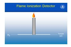
hydrocarbon analysis, with a detection range from 0.1ppm to almost 100%. The FID's response is stable from day to day, and is not susceptible to contamination from dirty samples or column bleed. It is generally robust and easy to operate, but because it uses a hydrogen diffusion flame to ionize compounds for analysis, it destroys the sample in the process.
